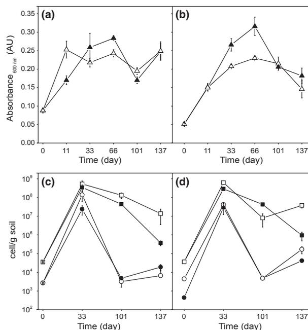
**Fig. 2.** Cell growth of consortia C2PL05 (a) and BOS08 (b) at high (25–15 °C; filled triangles) and low (15–5 °C; empty triangles) temperature range during PAH biodegradation; and MPN [cells (g soil)<sup>-1</sup>, fresh weight] for consortia C2PL05 (c) and BOS08 (d) of heterotrophic (squares) and PAH-degrading (circles) bacteria cultivated at high (filled symbols) and low (empty symbols) temperature range.
