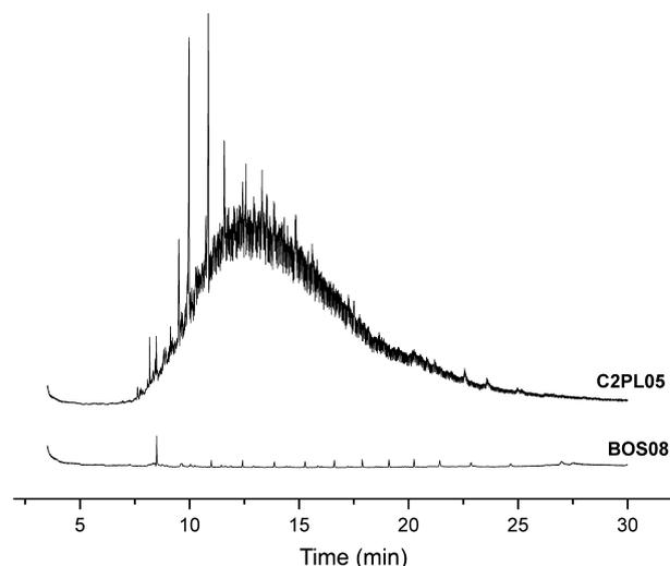
**Fig. 1.** Chromatogram showing TPH extracts from soils where consortia C2PL05 and BOS08 were isolated. The analysis was performed using a GC-flame ionization detector fitted with a Zebtron ZB-1XT capillary column. Helium was used as carrier gas.
