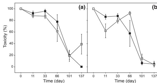
**Fig. 3.** Toxicity of microcosms with consortium C2PL05 (a) and BOS08 (b) incubated at high (25–15 °C; filled squares) and low (15–5 °C; empty squares) temperature range during PAH biodegradation process. Toxicity was measured using the Microtox assay, which measures the luminescence inhibition of *Vibrio fischeri*.
